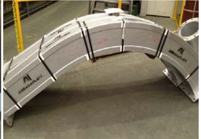
Chip Transfer Chute
