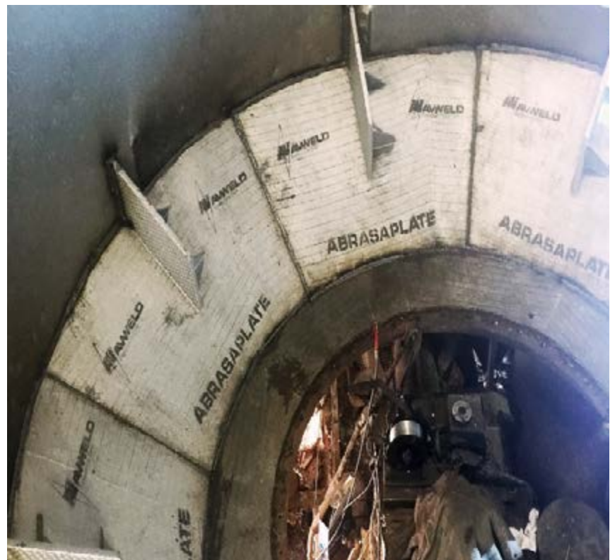
Hydropulper lined with AbrasaPlate wear plates, with AbrasaPlate-X cross hatch baffle plates
