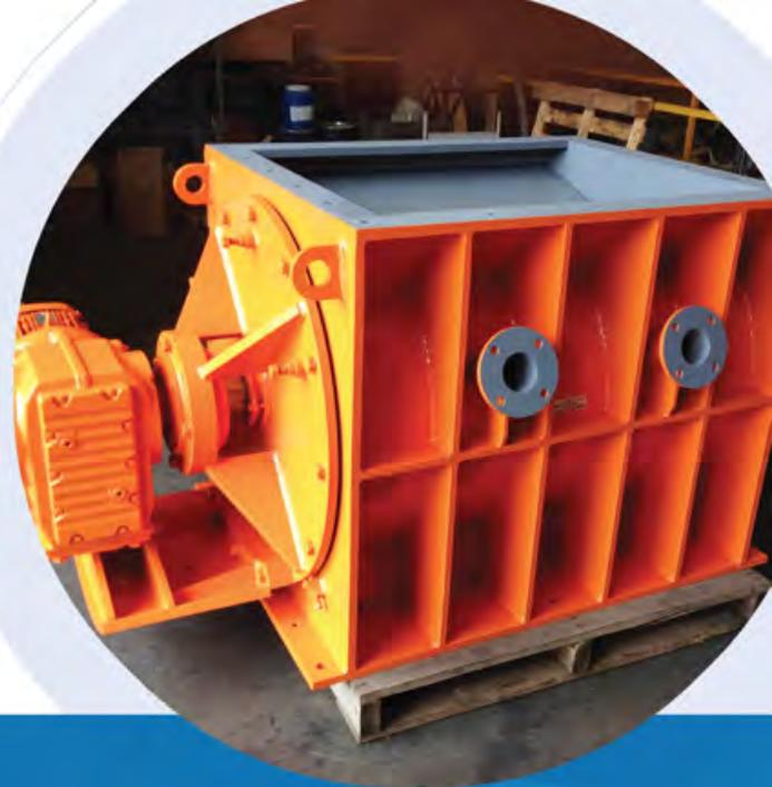
7. Tungsten Carbide coated packing gland journal. Allows use of hard or soft packing with no risk of wear again reducing maintenance and reducing by-pass.
