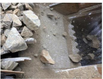
AP-X provides greater impact resistance than standard chrome carbide overlay plate.
