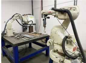
In addition, we are currently upgrading our existing gantry robotic facility with the same robot as above. As well as increasing the capacity this will ensure ease of operation and programming with all our cladding systems being based on ABB robots.
