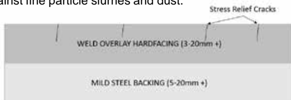
Cross section of AbrasaPlate
