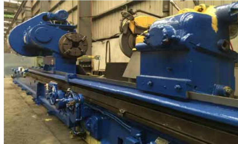
Cylindrical Grinding (1.8m diameter x 9m length)
