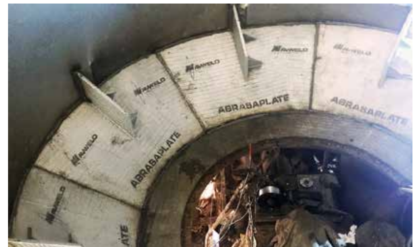
Hydropulper lined with AbrasaPlate wear plates, with AbrasaPlate-X cross hatch baffle plates
