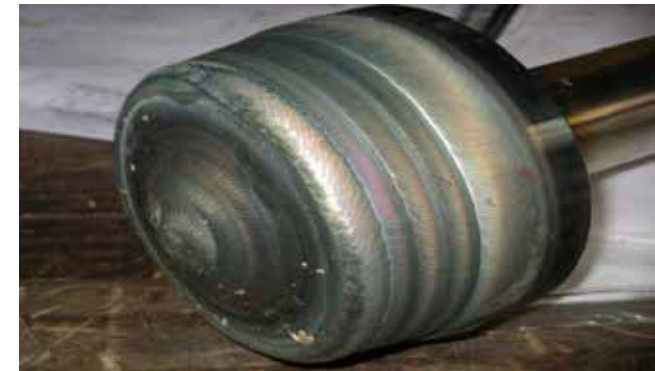
Valve-plug PTA welded with Stellite
