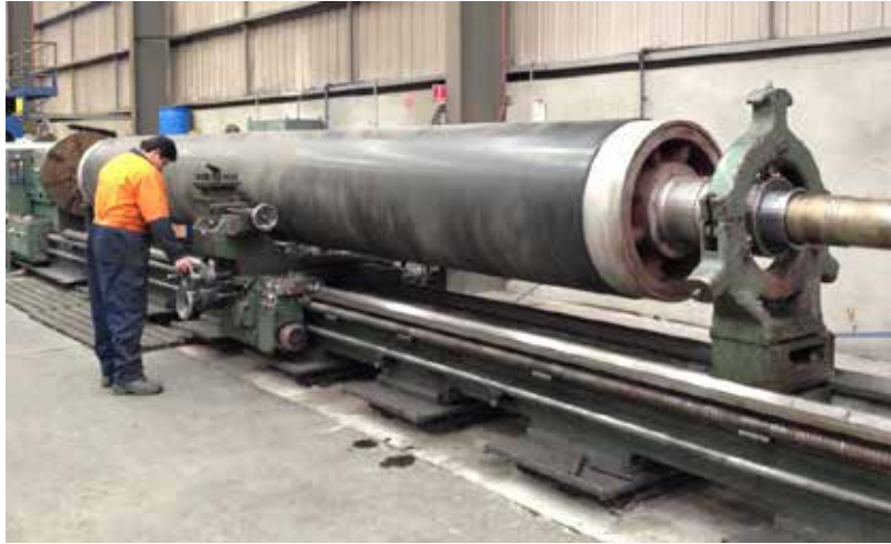
Machining (1.4m diameter x 11m length)
