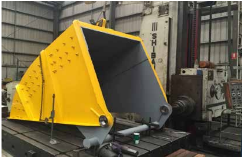
Horizontal Borer (Table 6m x 3m x 3m)
