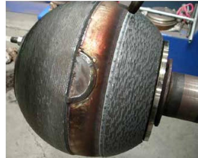
Robotically welded ball valve
