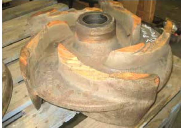
Above: Worn out pump impeller before repair.
