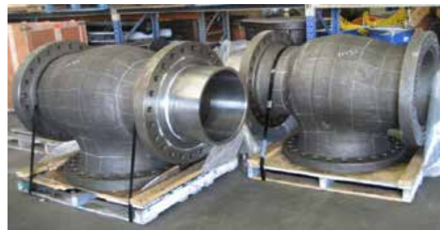
600mm Lunkenheimer Valve bodies ready for hardfacing with AV10™
