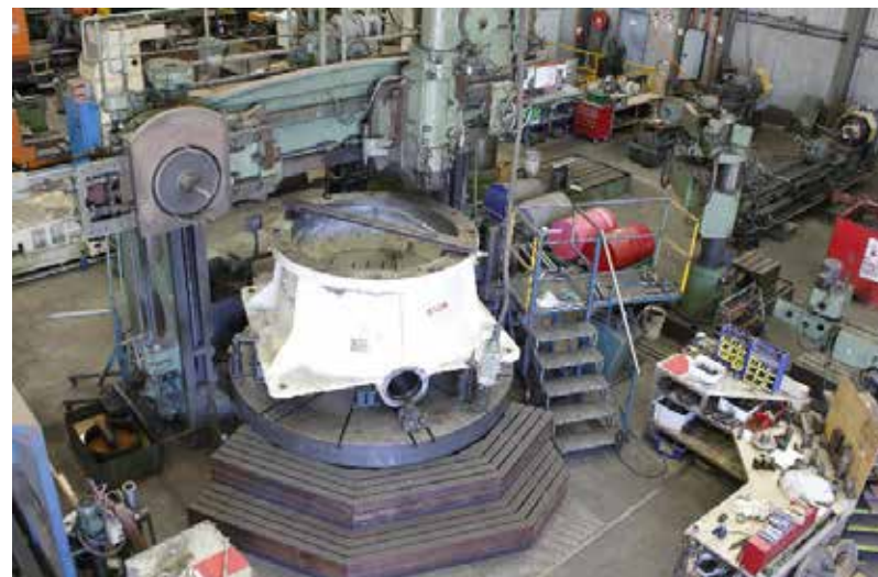
Large Vertical Borer – 3.5m diameter
