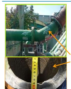
Internal pipe welding in the TBM is becoming the preferred wear resistant coatings above traditional Ceramic or Basalt, as in the past.
