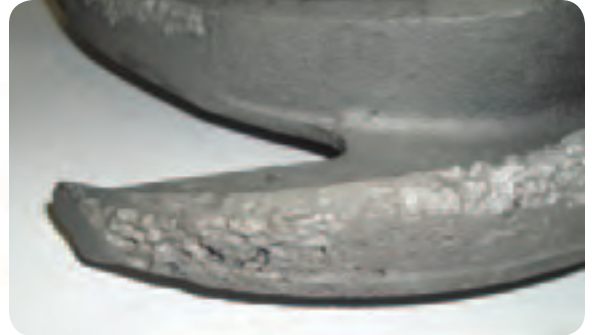
Worn impeller prior to repair.
